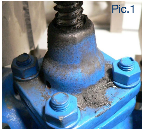
Pic. 1:Yakacik valve bonnet: Due to the high wear on the spindle thread, the valve test had to be terminated prematurely.
